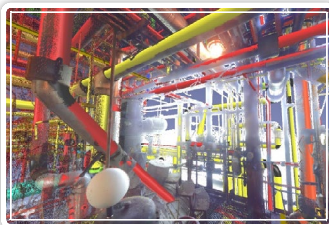
EdgeWise was able to accurately extract and model nearly 70% of the scanned pipes.
